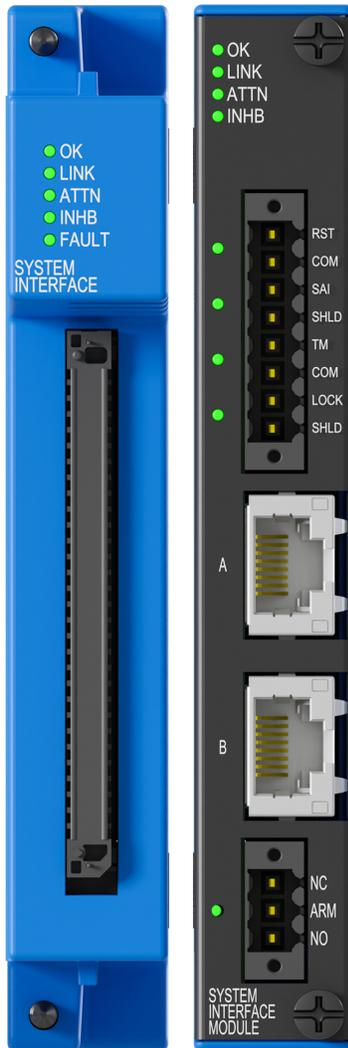
Each Orbit 60 system requires a single System Interface Module (SIM). The SIM provides the user access to manage protection configuration, local display, system-level diagnostics, system LEDs, system contacts, and the system protection fault relay. The SIM occupies one slot and must be adjacent to the Power Input Module (PIM) in the chassis.
