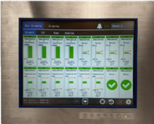
The Orbit Display system includes your choice of display screen, an industrial computer with a customized operating system, and software that communicates with one or more Orbit 60 systems. The system can be certified for hazardous locations. Condition monitoring data is communicated to external displays via a Display Port or VGA connection.
