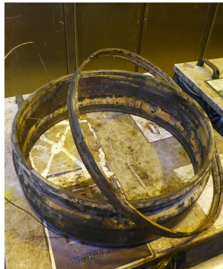
A modified version of the Baker Hughes MASTODON hydraulic pulling tool freed this shallow fish in a matter of mere minutes without any impact on surface equipment.
