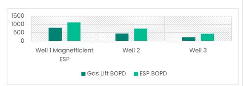
The operator's three wells experienced a 56 percent increase in production after conversion from gas lift to Baker Hughes Centrilift ESPs. The Magnefficient ESP with the new PMM safety module experienced the highest production increase.
