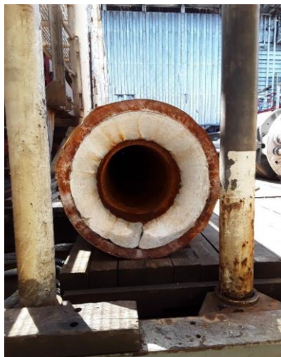
A 20 x 36-in. (0.812 x 2-in. WT) casing stump.
