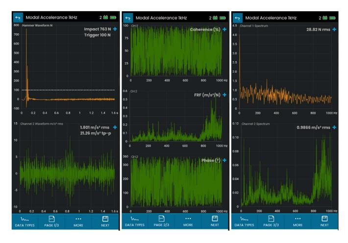
5. A comprehensive series of checks are automatically performed for each impact, with a composite Warnings message informing the user of any issues. Suggestions are provided for correcting each issue. Any of the 9 warning types can be Enabled, Paused or Disabled, if required.
