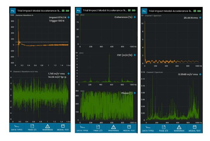
4. Performing actual Modal Impact Tests in Run mode and recording the specific locations and directions used.
