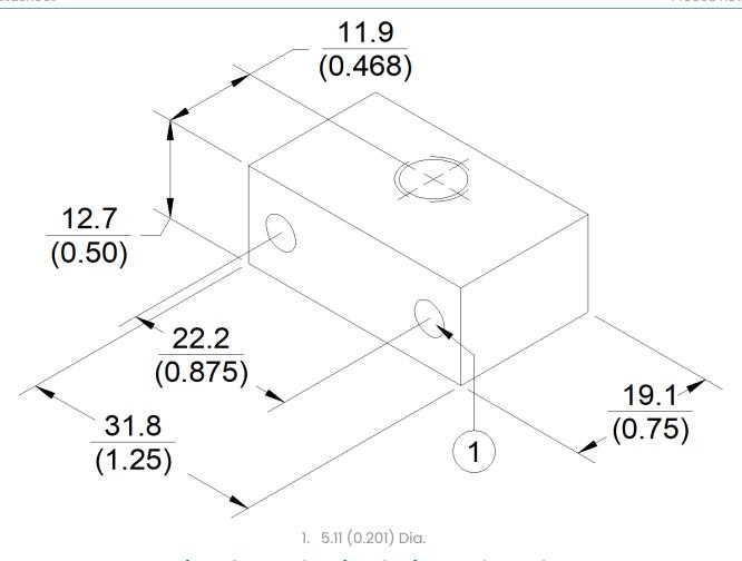
Figure 6: Non-Clamping Aluminum Probe Bracket
