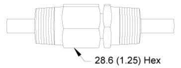
Figure 10: Low Pressure Cable Seal
