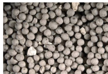
1% by weight ScaleSorb particles with 20/40 mesh proppant
