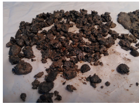
Samples of wellbore debris removed from the well by the PrecisionCollector 250
