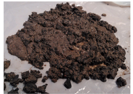
Samples of wellbore debris removed from the well by the PrecisionCollector 250
