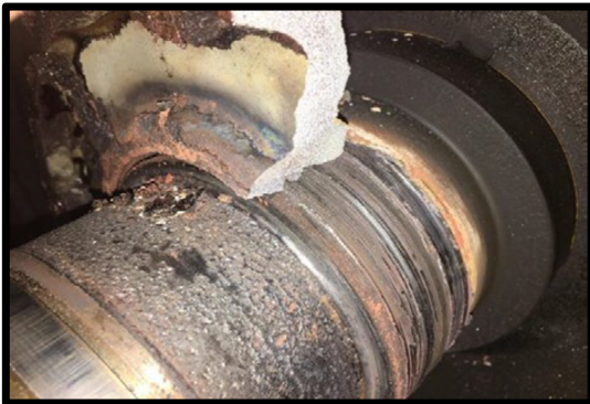
Figure 9 – Evidence of Motor Failure. Source: Eldorado Brasil Internal Files
