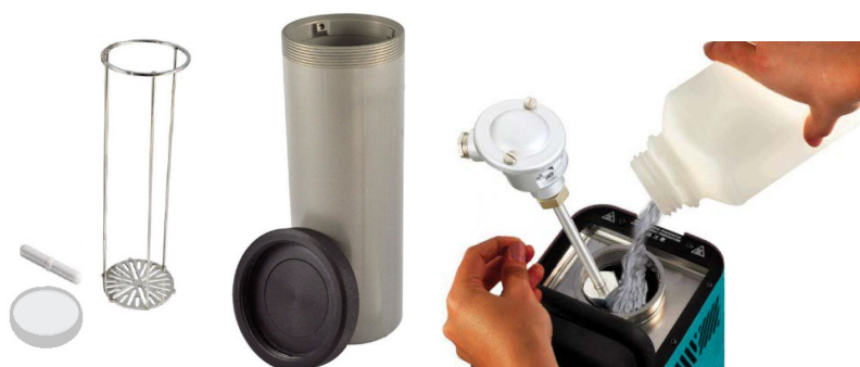
Figure 14: Filling with Calibration Liquid
