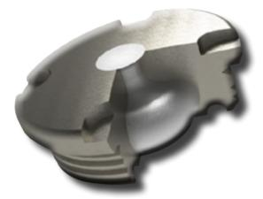
Once the liner is at planned setting depth, the reactivity of the IN-Tallic Damorphe can be triggered by spotting a wide variety of common completion brines, thus dissolving the material and allowing casing communication with the formation in a consistent and repeatable time window. Once the IN-Tallic Damorphe plug has dissolved, the stimulation treatment can be pumped through the assembly.
