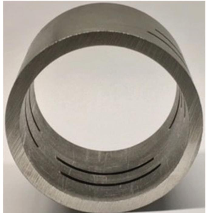
Pipe cut by the MPC InCision slot cutter.
