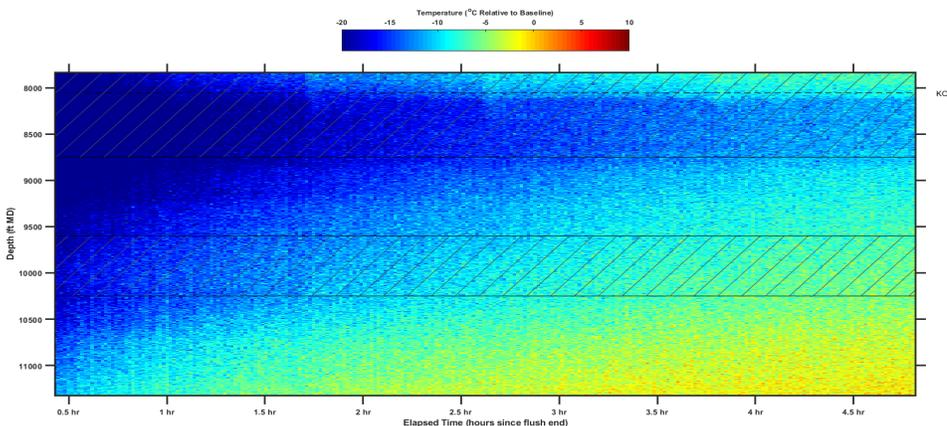
SureVIEW Coil post-stimulation DTS results show warmback temperature changes, aiding in the identification and optimization of acid and diverter placement.
