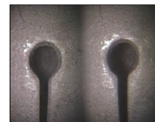
Good Example -- Object is: Fully visible on both sides. Well lit with minimal glare Oriented to allow placement of cursors at left and right edges of circle or gap
