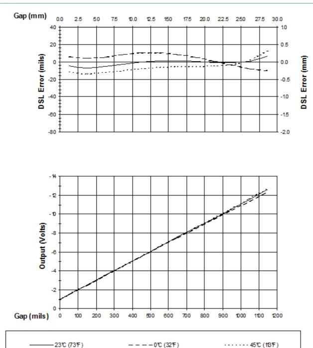
Figure 2: Typical 3300 XL 50 mm 9 m System Over Ambient Testing Range
