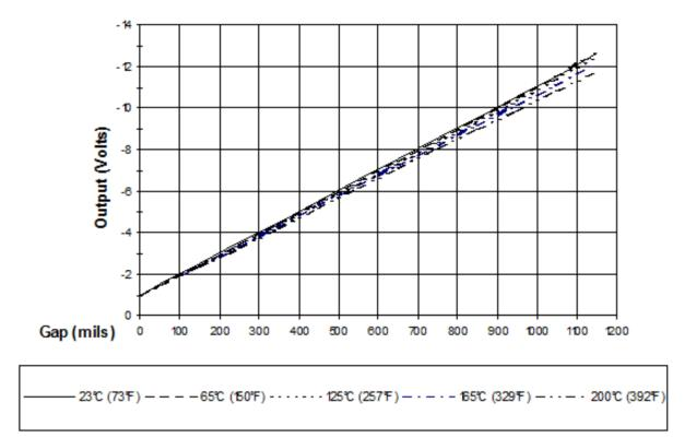
Figure 4: Typical 3300 XL 50 mm Probe + 1m Cable @ High Temperature (Proximitor Sensor + 8m of Extension Cable @ 25 °C)
