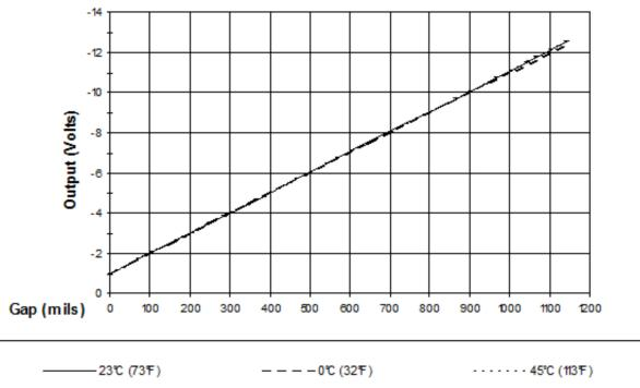
Figure 1: Typical 3300 XL 50 mm 5 m System Over Ambient Testing Range
