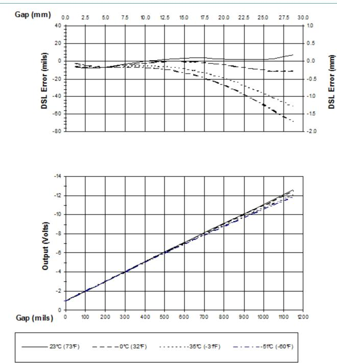
Figure 7: Typical 3300 XL 50 mm 9 m Proximitor Sensor with 8 m of Extension Cable @ Low Temperature (Probe is at 25°C)
