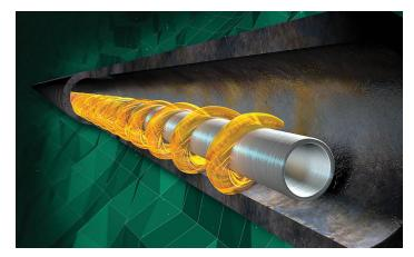
EasyReach lubricant can reduce the coefficient of friction by as much as 60% in downhole conditions, helping extend the reach of coiled tubing in long wellbores.
