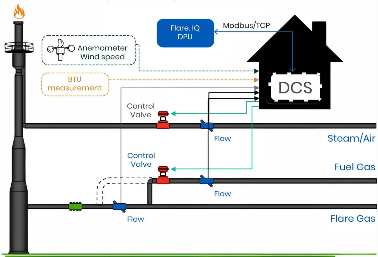
**Figure 1: Schematic of flare.iQ-based control of flare assist (Steam/Air) and supplemental fuel**
