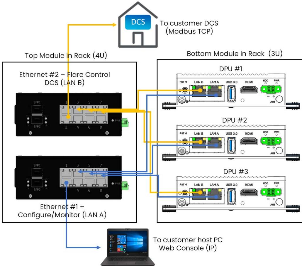
**Figure 36: System I/O network connections**
