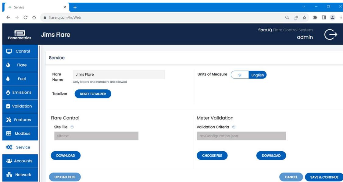
Figure 17: Service configuration page that enables uploading installation specific site files
