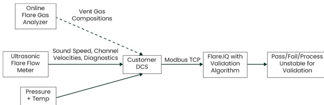
**Figure 9: Digital Flare flow meter validation scheme**
