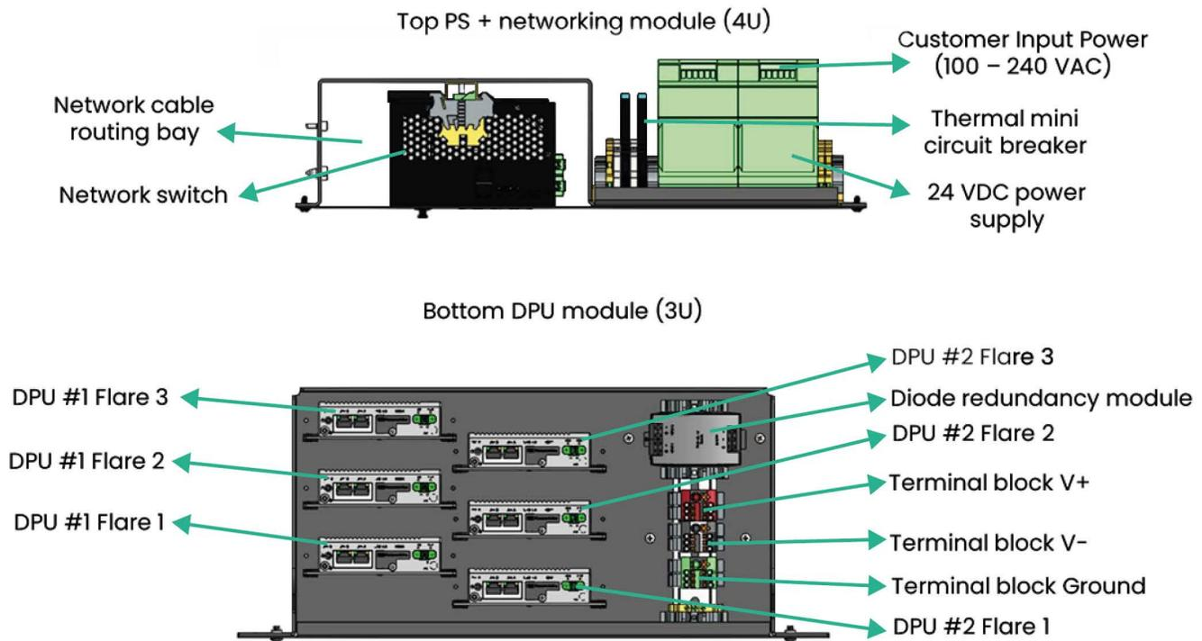
**Figure 38: Recommended module and DPU placement (primary #1 and redundant #2 for each flare)**
