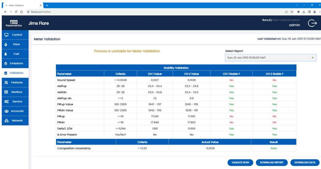
**Figure 29: Validation page showing results of an unsuccessful digital verification due to process instability.**
