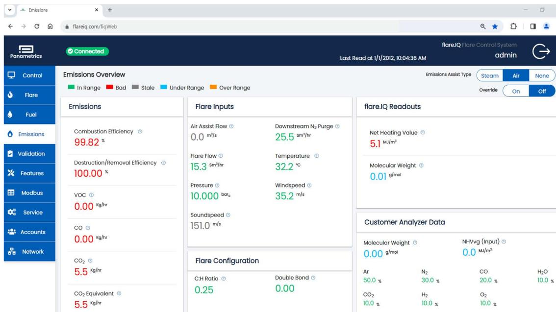
**Figure 30: Emissions page without Modbus connection**
