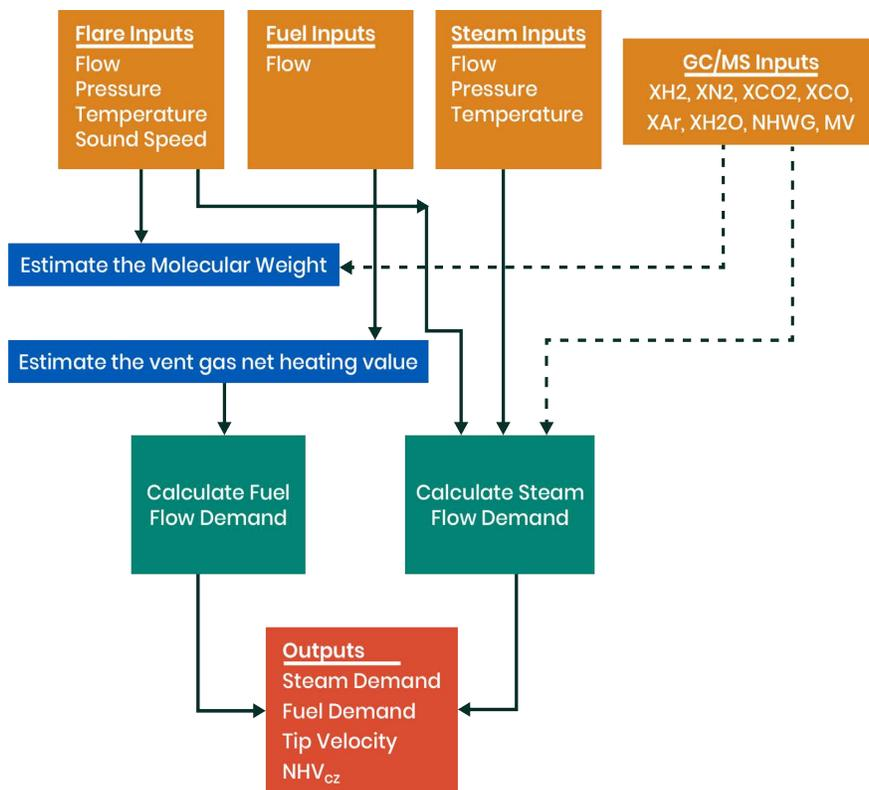
Figure 8: High-level flare control process logic flow
