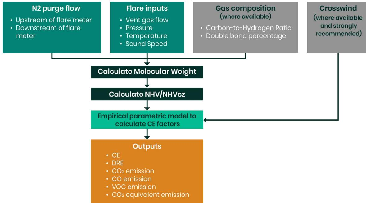
**Figure 11: High-level schematic of flare CE, DRE and emissions calculations**
