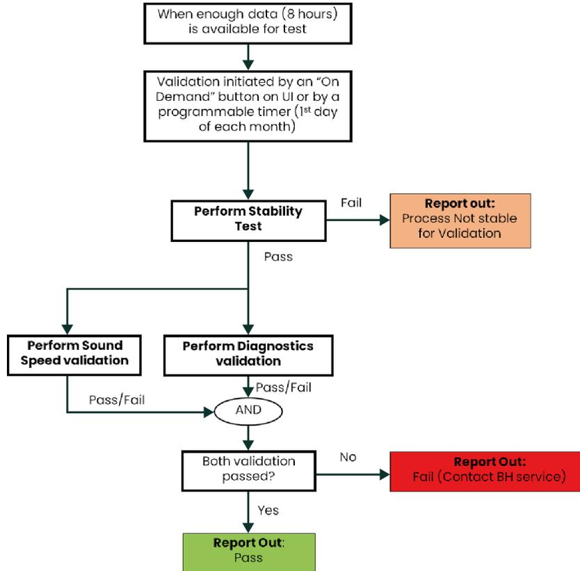
**Figure 10: Flare flow meter validation logic**
