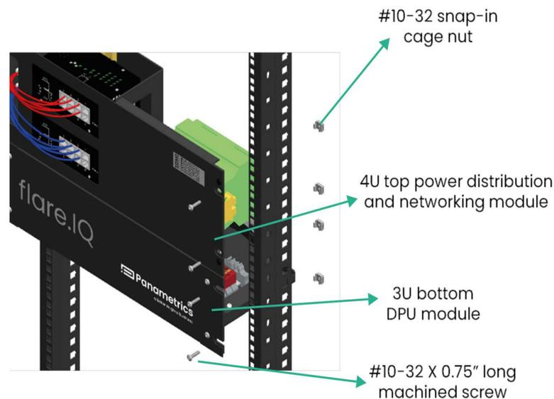
**Figure 37: Recommended rack mounting method**
