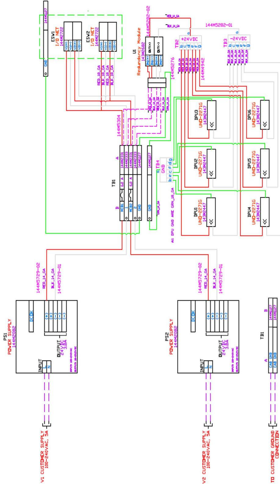
Figure 35: System Wiring Diagram
