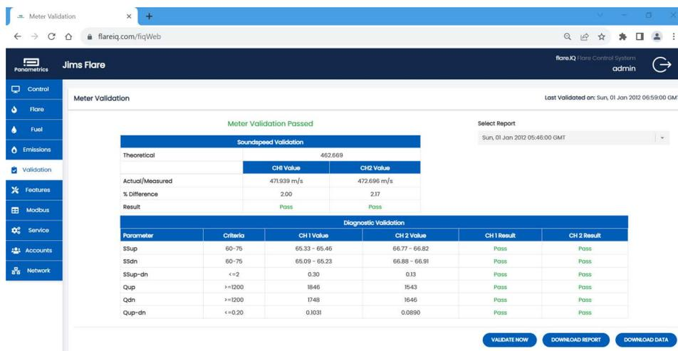
**Figure 28: Validation page showing typical result for passing digital verification**
