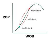
Critical to optimizing rotational based wellbore cleanout operations is the ability to provide the required parameters of torque, weight on bit (WOB) and RPM combined with a specifically designed bit and augur system, in turn delivering optimized rate of penetration (ROP) throughout the task at hand.
