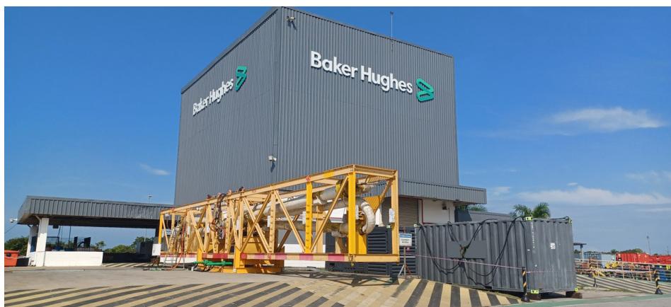
Flow test plant located at Rio de Janeiro–Brazil with one ESP Subsea Boosting System under testing.
