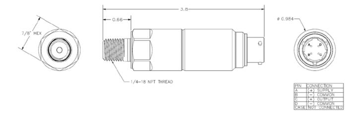
Figure 1: 350300 Dynamic Pressure Sensor Dimensions and Pinout
