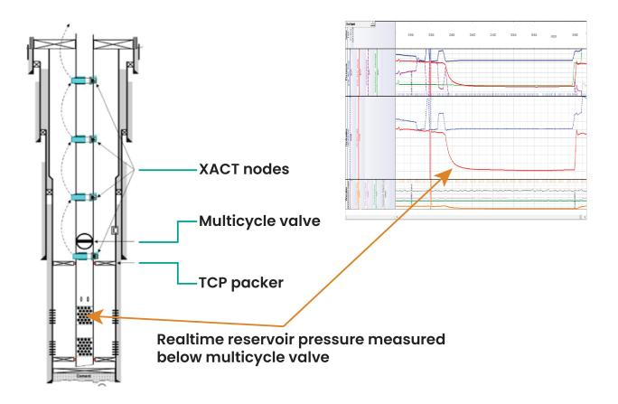
XACT tools positioned along the worksting and below a multicycle valve provide realtime downhole reservoir pressures during perforation operations.
