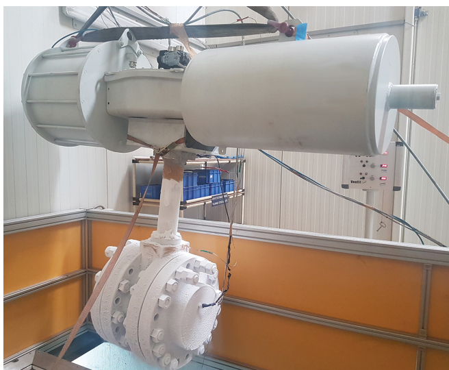
Figure 1. Triple eccentric butterfly valve performing leakage tests using nitrogen.
