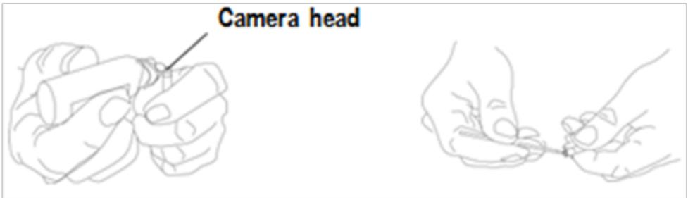
**2** – Clean all external parts of the camera head. Use glass cleaner or 70% alcohol-to-water solution and a pointed cotton swab.
