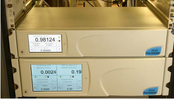
Picture 1: PACE5000 and PACE6000 modular pressure controllers
