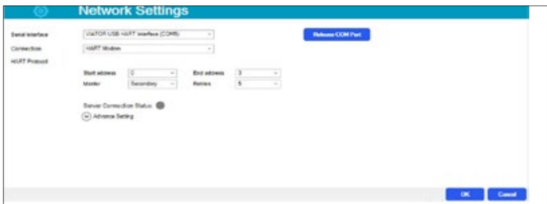
The screenshot shows the 'Network Settings' dialog box. The 'Serial Interface' is set to 'VALTOR USB HART Interface (COM6)'. The 'Connection' is set to 'HART Modem'. Under 'HART Protocol', the 'Start address' is 0, 'End address' is 3, 'Master' is 'Secondary', and 'Parity' is '5'. There is a 'Release COM Port' button at the top right. At the bottom right, there are 'OK' and 'Cancel' buttons.
