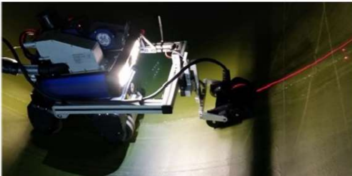
Figure 5: Bike with EC array probe inspecting the inside of a tank
