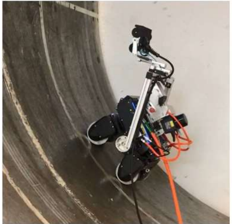
Figure 4: Bike with EC array probe rolling up the inside of cylindrical tank
