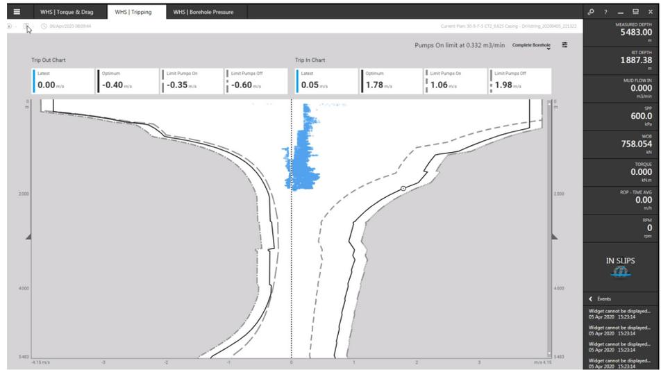
The user interface for the i-Trak Tripping Advisor adapts dynamically and automatically to current operational conditions—allowing simple, intuitive parameter identification to alleviate ILT and ensure borehole integrity.
