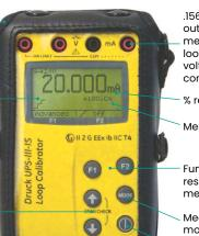
.156 in (4 mm) input/ output sockets: mA measure and source, loop power supply, voltage measure, continuity test
