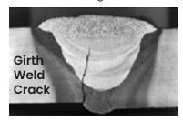
Girth weld failures are usually a combination of interacting threats, comprising of axial loading (from ground instability or thermal loads), defects within welds (weld cracks, anomalies or corrosion attack) and material (substandard weld material properties).
