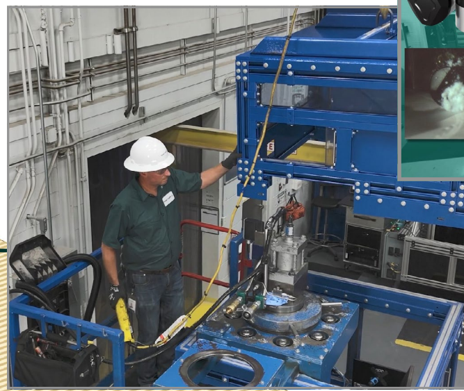
The visual single-point cutter machine details cutter/rock interaction during drilling at high pressures. Its unique perspective brings fresh ideas to cutting-edge technology and drilling efficiency.
