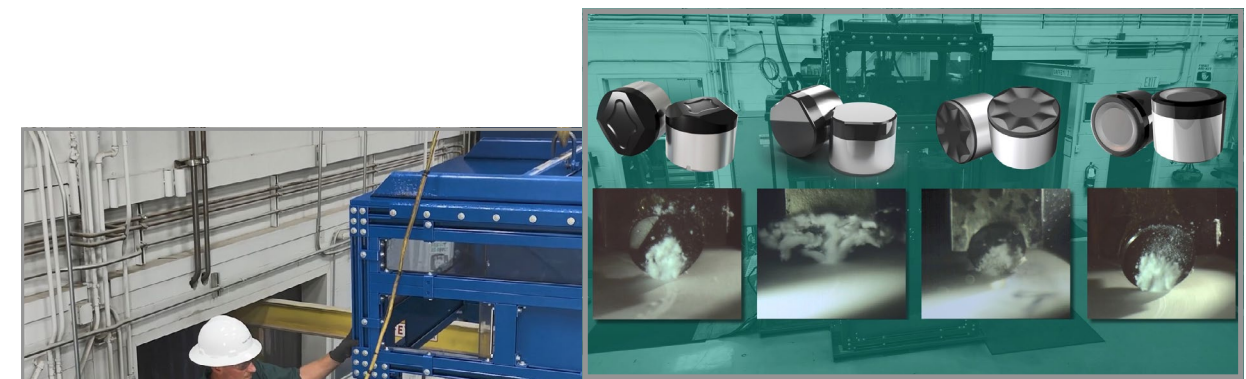
The visual single-point cutter machine details cutter/rock interaction during drilling at high pressures. Its unique perspective brings fresh ideas to cutting-edge technology and drilling efficiency.
