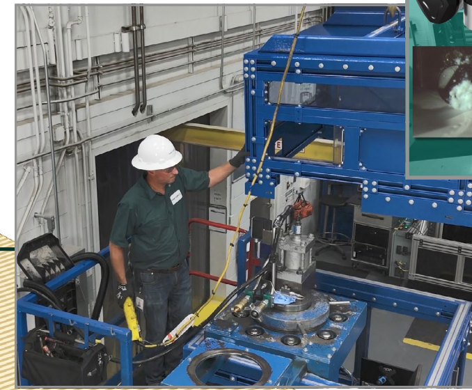
The visual single-point cutter machine details cutter/rock interaction during drilling at high pressures. Its unique perspective brings fresh ideas to cutting-edge technology and drilling efficiency.
