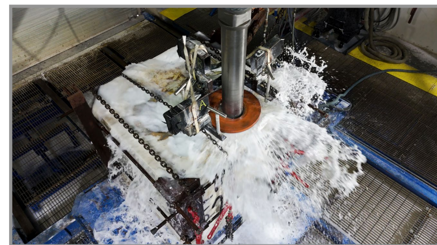
Our full-scale atmospheric pressure test rig facilitates dynamic analysis of all types of drill bits.
