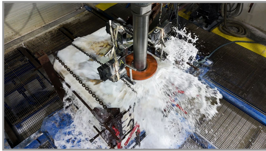
Our full-scale atmospheric pressure test rig facilitates dynamic analysis of all types of drill bits.
