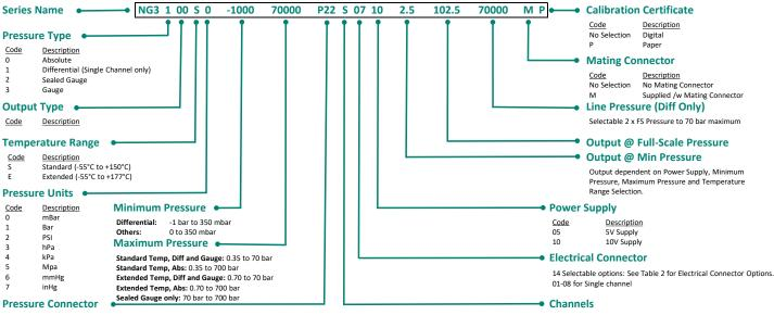
12 Selectable options. See Table 1 for Pressure Connector Options. Pressure Type: 1 – Side port pressure connector auto selected to match front port selection.
