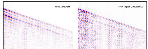
This side-by-side comparison shows a raw vertical seismic profile (VSP) shot point acquired above the well (left) versus VSP from 43 miles (69 km) from the wellhead (right). The "local" (left) case uses CoreBright only. The "remote" (right) case uses a 69km CoreBright lead-in, 3dB attenuation and subsea amplifier, and CoreBright EBF inside the well.
