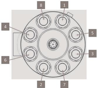
Figure 1 - Torque Sequence Single Bolting Circle 8 Bolts
