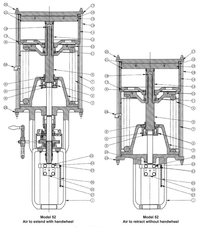
Figure 12: Model 52 Actuator
