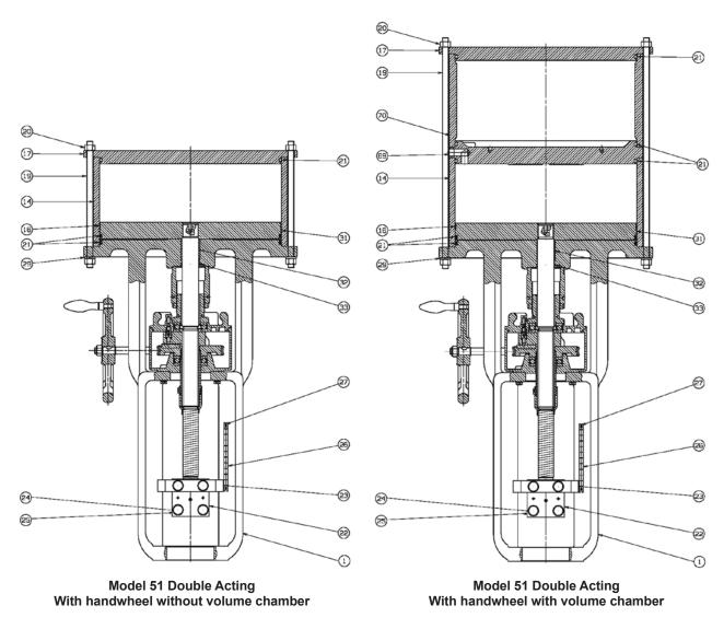
Figure 10: Model 51 Actuator
