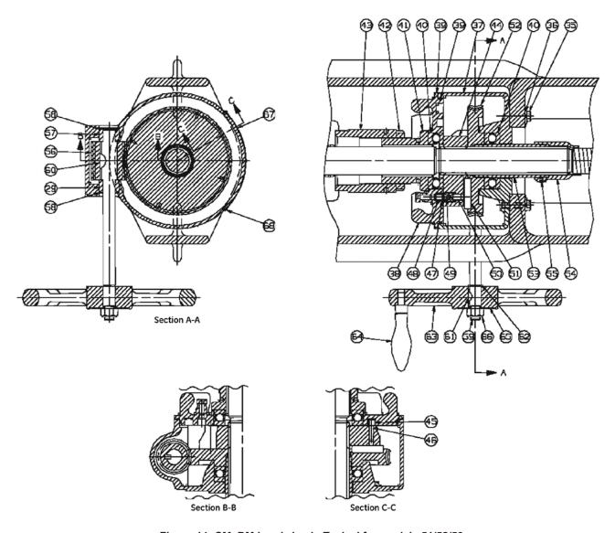
Figure 14: CM, DM handwheel - Typical for models 51/52/53
