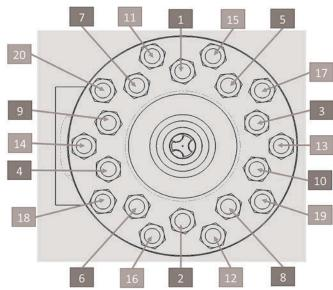
Figure 4 - Torque Sequence Single Bolting Circle 20 Bolts
