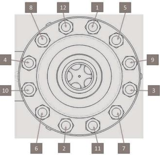
Figure 2 - Torque Sequence Single Bolting Circle 12 Bolts
