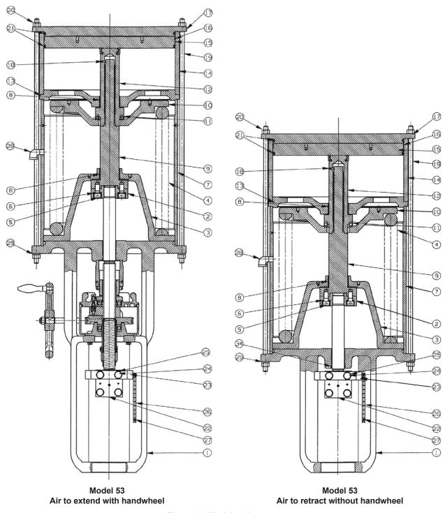
Figure 13: Model 53 Actuator
