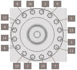
Figure 3 - Torque Sequence Single Bolting Circle 16 Bolts
