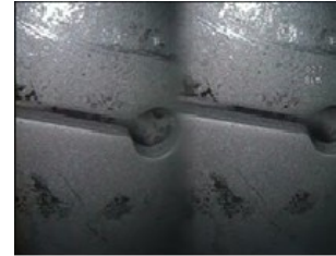
Bad Example -- Object is: Not fully visible on right side. Not well lit (optical tip needs to move closer to surface) Not oriented to allow placement of cursors at left and right edges of circle or gap
