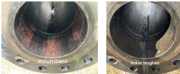
Copper Ion displacement testing in spool with incumbent corrosion program (left) and Baker Hughes corrosion program (right)
