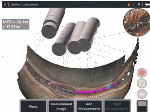
3D Stitching on tube inner bore diameter measurement
