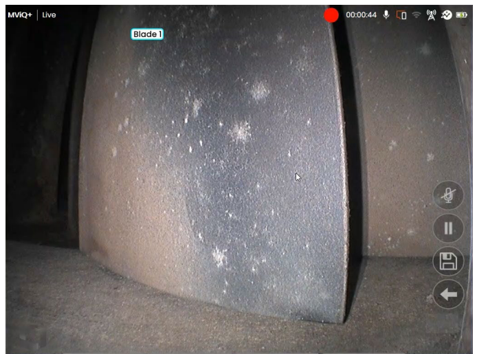
Figure 9. Blade Counter active showing blade number text box.
