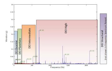
Finally, a DEI multiplier is used to produce a number that is easier to use. DEI values have no physical meaning in and of themselves; they are used to trend vibration levels over time. To summarize, DEI is calculated through a number of steps. For each DEI band;
