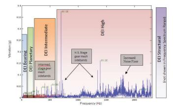
Each DEI band value can be independently alarmed and trended, and alarms can be set independently for different wind turbine power bands (modes). In ADAPT Wind, it is possible to set a total of 25 DEI alarms, five for each power mode times five DEI bands.
