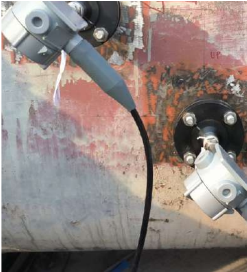
T5 Bias 90 installation with XAMP preamplifiers on the 64" (DNI600) line
