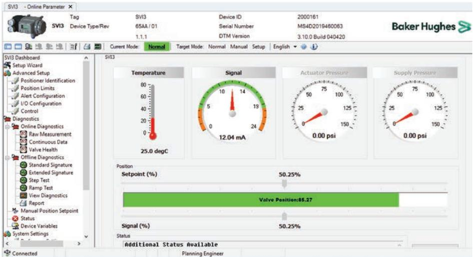
2. For device configuration, the SVI3 should be in the **Setup** mode. Click **Setup** in the DTM screen to switch the device into Setup mode.
