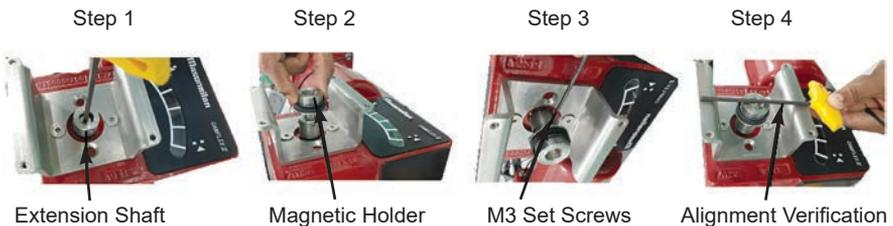
Figure 4 - Mounting Kit Assembly Procedure on Rotary Valve
