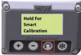
2. Release the button for Calibration
