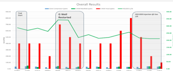
FullSweet HSS1003 cost-effectively lowered H 2 S-associated corrosion with no adverse effects on gas compressors.
