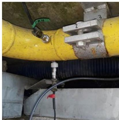
Fig 12: Monoaxial sensors positioning
