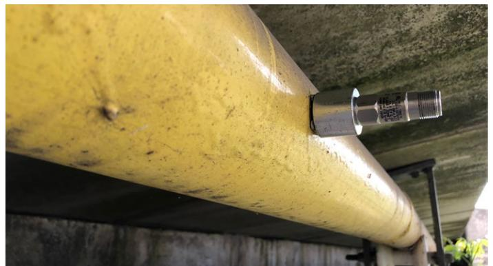
Fig 5: Example of temporary magnet based installation of the sensor
