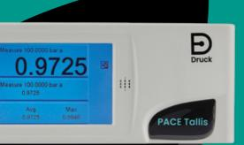
Druck's ADTS pitot static testers require accurate calibration to ensure RVSM compliance. Traditionally, users need to send their ADTS for servicing, meaning a loss of operation when in transit. Using PACE Tallis as a portable, in-house calibrator reduces calibration time to a matter of hours, as opposed to weeks.
