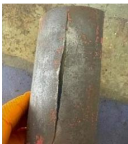
Rod cracking and splitting due to high friction prior to treatment
