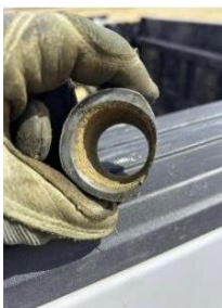
Rod cracking and splitting due to high friction prior to treatment
