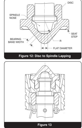
out. Place a ring lap on a table, or similar flat surface, and wipe the exposed surface of the lap clean. Insert the disc nose into a ring lap, so that the seat contacts the lap surface. Oscillate the spindle using 360-degree oscillations for approximately 15 seconds, then check the spindle tip and disc "pocket" to determine progress. (See Figure 11.)
