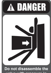
Do not disassemble the valve with pressure in the drum or header, as this will result in severe personal injury or death.
