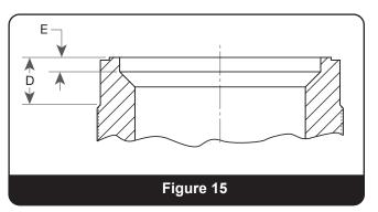
(ii) Lap, using an oscillating motion in various directions, while holding the lap loosely in the fingers and allowing the weight of the lap to rest on the seat surface. Control the motion of the lap to prevent either the inside or outside edge of the lap from crossing the bushing seat surface. If either edge touches the seat surface, the seat can become scratched and/or rounded.
