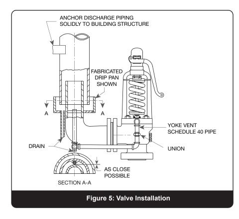
For optimum performance, safety valves must be serviced regularly and otherwise maintained. So that servicing can be properly performed, valves should be located in a manner that allows for easy access. Sufficient working space should be provided around and above the valve to permit access to adjusting rings. If two or more valves are located close together, the outlets should be parallel so as to offer as much protection as possible to personnel repairing, or working close to, the safety valve.
