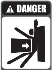
Do not disassemble valve with pressure in drum or header, as this will result in severe personal injury or death.
