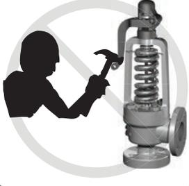
Improper tools or improper use of right tools could result in personal injury or product damage.
