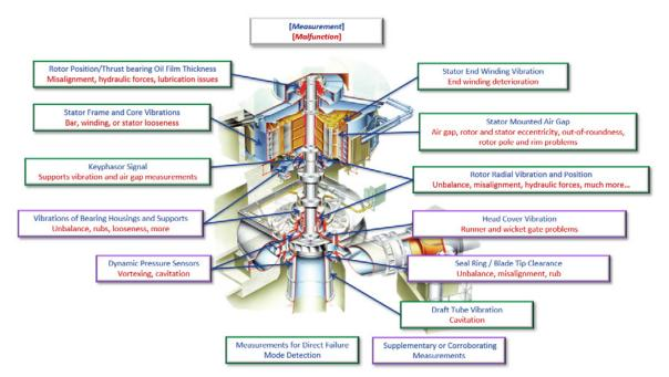
Figure 2: typical measurements and some corresponding malfunctions
