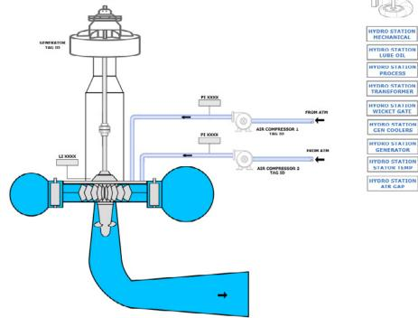
Figure 6e: diagnostic HMI of hydro air injection system
