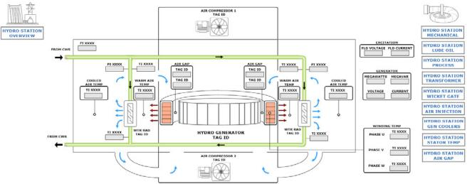
Figure 6c: diagnostic HMI of hydro generator
