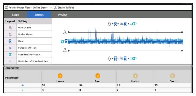
Figure 4: System 1 alarm quick configuration dialog box
