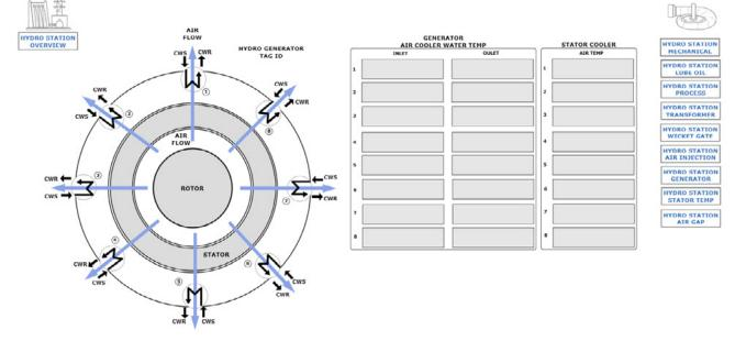
Figure 6g: diagnostic HMI of hydro generator coolers
