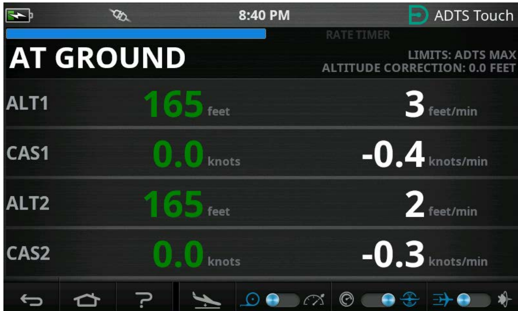
Figure 3-27: Go To Ground Complete – Multi Channel
