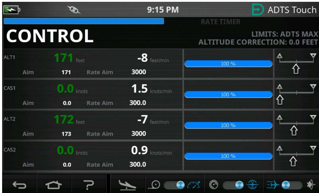
Figure 3-8: Control Mode – Multi Channel
