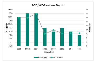
DYNAFLOW DIF provided excellent controls on ECD at different WOBs while drilling the section.
